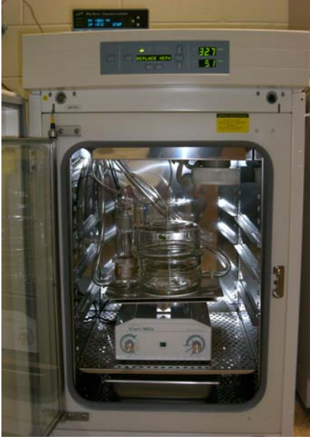
Figure2. Photograph of facility for exposing cell to Cl 2 . A glass exposure chamber is sitting on a platform rocker (bottom) and can be tilted during exposure. The heating mantle and air/gas humidifier are shown in the left of the glass chamber. The glass door is closed during exposure. The two tygon tubes from the sides of the chamber vent to the inside of a nearby Biosafety Level Two hood.
